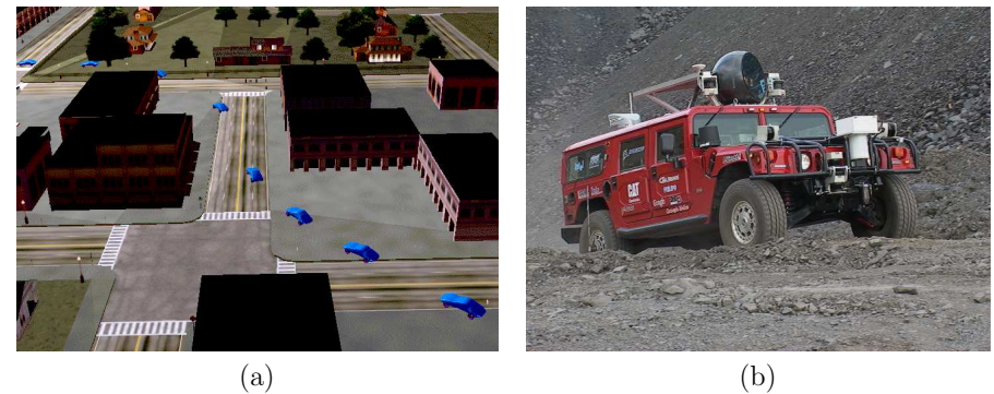
Figure 1.13: Reckless driving: (a) Using a planning algorithm to drive a car quickly through an obstacle course [199]. (b) A contender developed by the Red Team from Carnegie Mellon University in the DARPA Grand Challenge for autonomous vehicles driving at high speeds over rugged terrain (courtesy of the Red Team).
