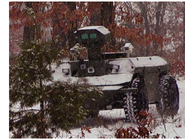
Figure 12.17: The Automated Cross-Country Unmanned Vehicle (XUV) is equipped with laser radar and other sensors, and uses Stentz's algorithm to navigate (courtesy of General Dynamics Robotic Systems).
