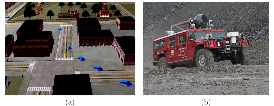
Figure 1.13: Reckless driving: (a) Using a planning algorithm to drive a car quickly through an obstacle course [4]. (b) A contender developed by the Red Team from Carnegie Mellon University in the DARPA Grand Challenge for autonomous vehicles driving at high speeds over rugged terrain (courtesy of the Red Team).
