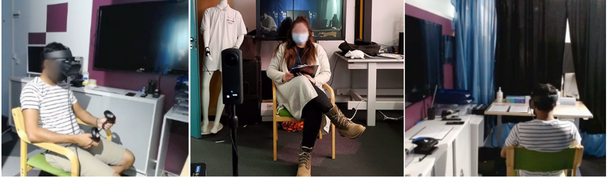
Fig. 1: Head-mounted display telepresence augmented with a virtual body; the participant (side images) is sitting in one place wearing a head-mounted display, but is telepresent in another location through a live streaming camera having a discussion with an experimenter (center image) and can see robot arms in one condition that match their real arms' motions.
