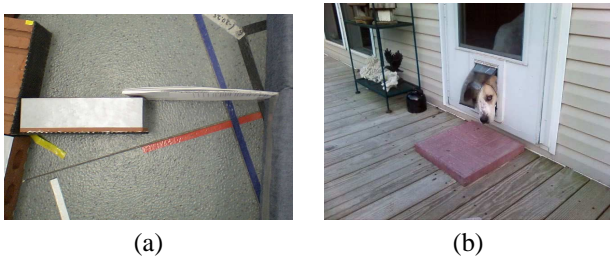
Fig. 4. a) A static, directional gate can be implemented making a flexible “door” from a stack of paper; in this case, the body can transition only from the bottom region to the top; b) this works much like a “doggie door”.
