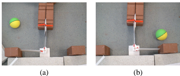
Fig. 10. A gate with two modes: a) a ball can pass from left to right, but its blocked the other way; b) a ball can only pass from right to left.
