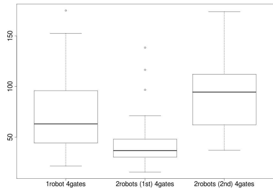
Fig. 15. Plot of completion times (seconds) for one robot (left), two robots first arrival (middle), two robots second arrival (right)
