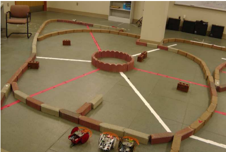
Fig. 2. An annulus-shaped environment that has 6 regions. The walls are made of bricks and the virtual gates are made of colored tape. There are three RED gates and three WHITE gates.
