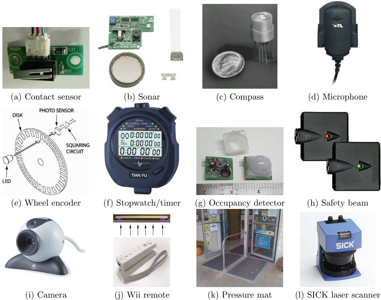
Figure 4: Some examples of widely available sensors, roughly sorted from low-cost to high-cost.
