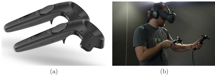
Figure 10.12: (a) A pair of hand-held controllers that came with the HTC Vive headset in 2016; the device includes side buttons, a trigger, and a touch pad for the thumb. (b) A user trying the controllers (prototype version).
