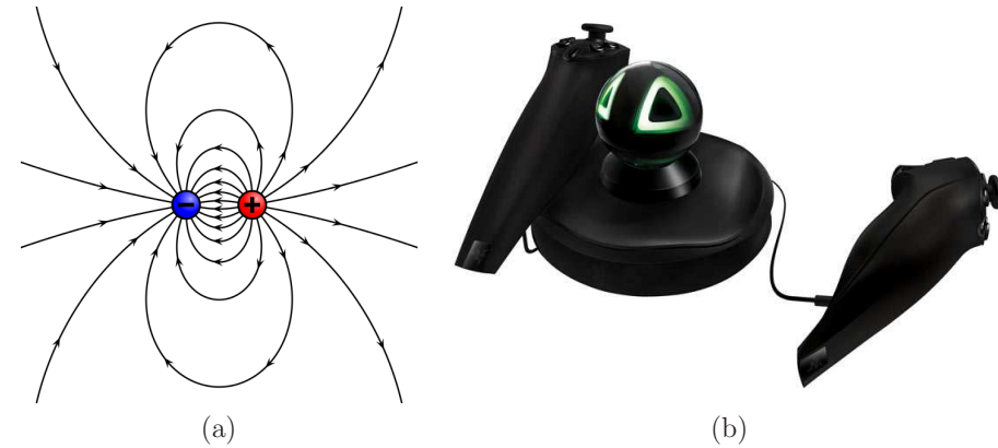
Figure 9.10: (a) A magnetic dipole offers a field that varies its magnitude and direction as the position changes (figure by Wikipedia user Geek3). (b) The Razer Hydra, a game controller system that generates a weak magnetic field using a base station, enabling it to track the controller positions (figure by http://www.GamingShogun.com/ ).
