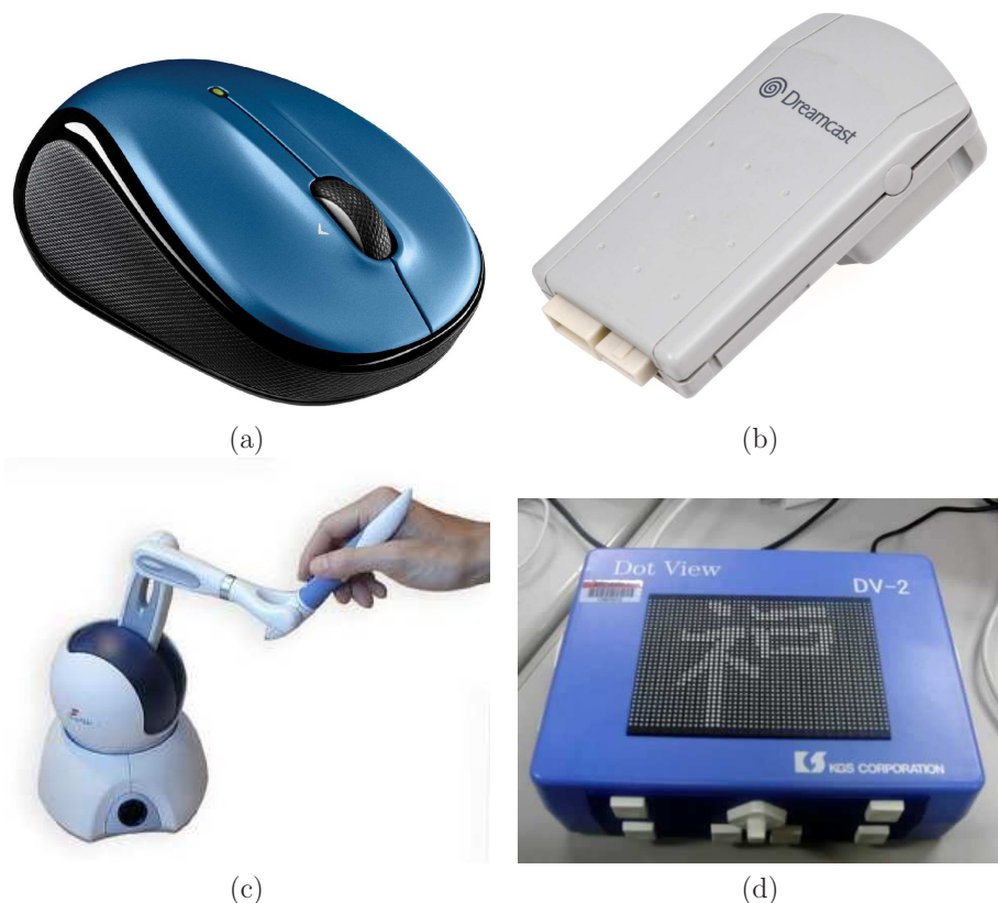
Figure 13.4: (a) The Logitech M325 wireless mouse with a scroll wheel that provides tactile feedback in the form of 72 bumps as the wheel performs a full revolution. (b) The Sega Dreamcast Jump Pack (1999), which attaches to a game controller and provides vibrations during game play. (c) Haptic Omni, from 3D Systems, a pen-guiding haptic device, which communicates pressure and vibrations through the pen to the fingers. (d) The KGS Dot View Model DV-2, which is a haptic pin array. The pins are forced upward to simulate various textures as the finger tip scans across its surface.
