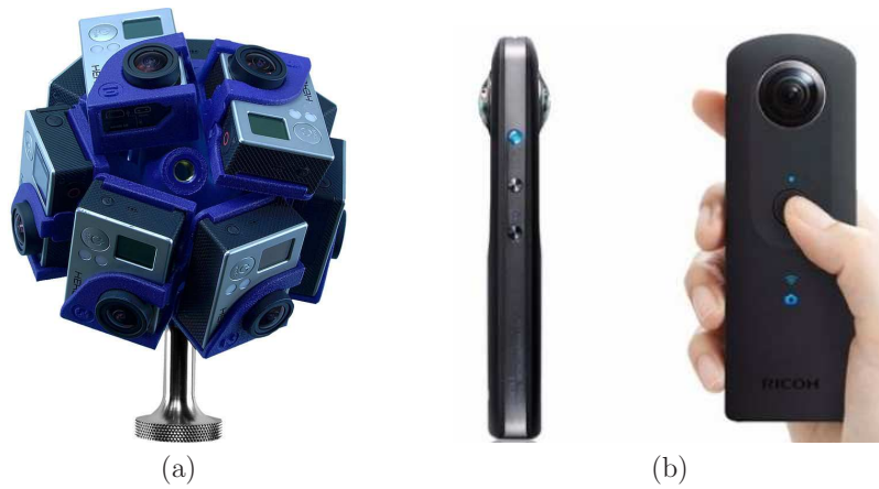
Figure 7.23: (a) The 360Heros Pro10 HD is a rig that mounts ten GoPro cameras in opposing directions to capture panoramic images. (b) The Ricoh Theta S captures panoramic photos and videos using only two cameras, each with a lens that provides a field of view larger than 180 degrees.
