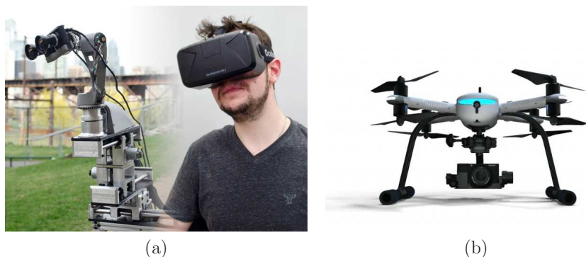
Figure 1.12: Examples of robotic avatars: (a) The DORA robot from the University of Pennsylvania mimics the users head motions, allowing him to look around in a remote world while maintaining a stereo view (panoramas are monoscopic). (b) The Plexidrone, a flying robot that is designed for streaming panoramic video.
