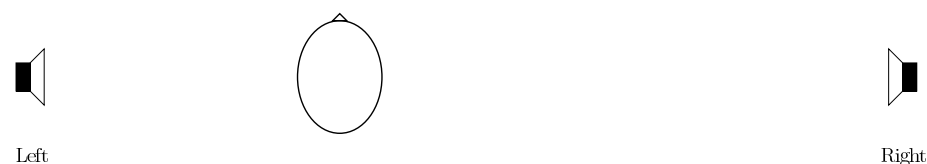
Figure 11.7: Due to the precedence effect , an auditory illusion occurs if the head is placed between stereo speakers so that one is much closer than the other. If they output the same sound at the same time, then the person perceives the sound arriving from the closer speaker, rather than perceiving an echo.
