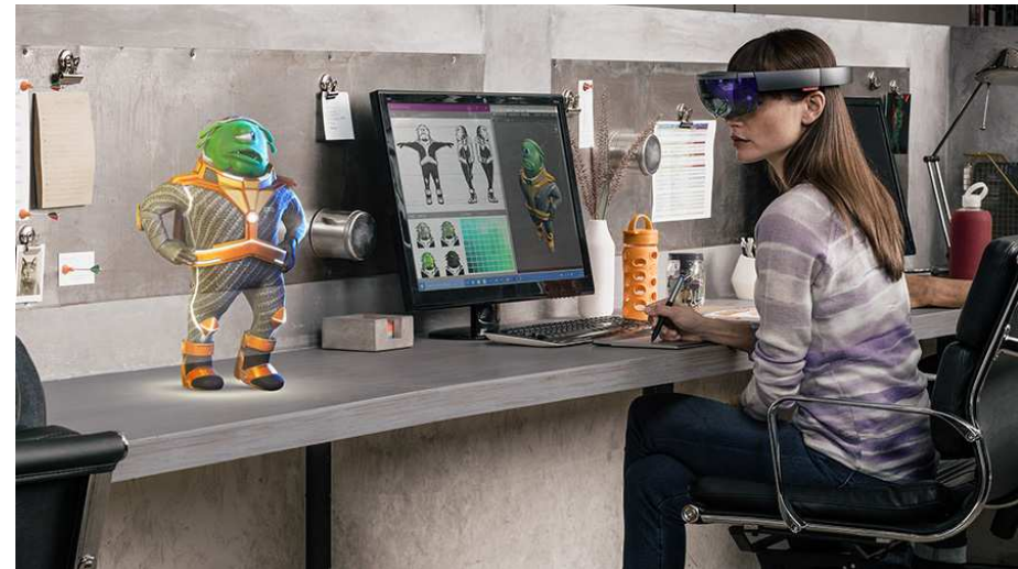
Figure 1.20: The Microsoft HoloLens, 2016, uses advanced see-through display technology to superimpose graphical images onto the ordinary physical world, as perceived by looking through the glasses.
