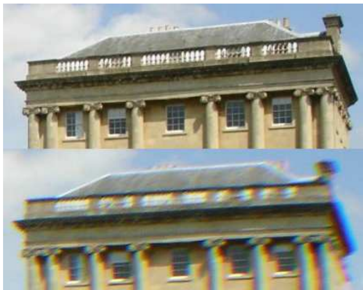
Figure 4.18: The upper image is properly focused whereas the lower image suffers from chromatic aberration. (Figure by Stan Zurek, license CC-BY-SA-2.5.)
