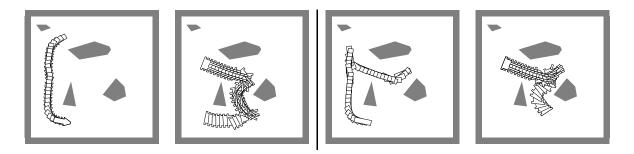
Figure 11: Two of five minimal quotient strategies for a two-robot problem with rotation.
