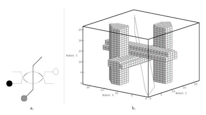
Figure 4: A coordination space for a three-robot fixed-path problem.
