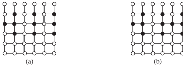
Fig. 1 Examples of the escape problem on a 6 \times 6 grid. The black discs are the initial evader locations. The goal is to plan disjoint paths for the evaders to reach different vertices on the boundary of the grid. a) An instance with solution given as the bold edges. b) An instance without a solution.
